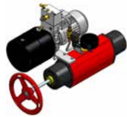
El-hydraulisk Aktuator Body Anodisert Aluminium Spring Return (SR) F07 – F16 Torque output | max. 5.000Nm Spindel SQR 17 - 46
