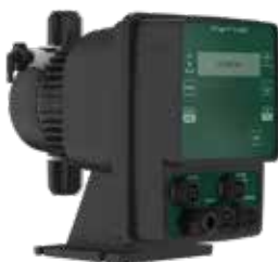
Solenoid drevet pumpe Flow rate | 2.5 – 110 l/h Mottrykk | Maks 20bar Stroke | 120 – 300 pr. min Membran | PTFE Pumpe hus | PVDF
