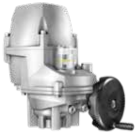
Elektrisk Aktuator AUMA Profox Multi-turn | Part-turn ISO 5211 Monteringsflens On/Off | 4-20mA Torque output | max. 600Nm
