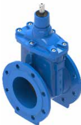
Sluseventil V2-05NT Myktettende EPDM Body EN-GJS-400-15 Ratt | Spindelforlenger | Aktuator DIN Flens DN40 – DN350
