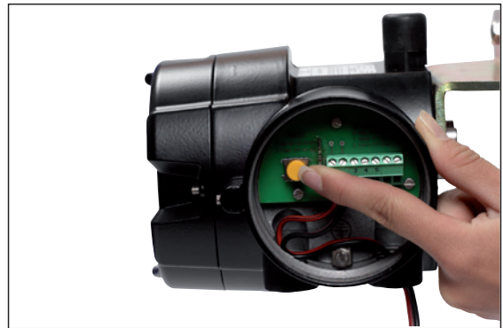
Press button and D20 will auto calibrate itself.
