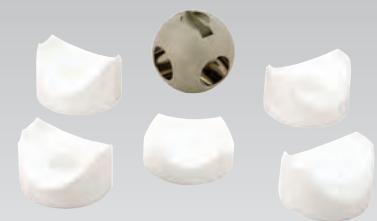
The cavity filled seats are designed to fill the dead space between the ball and valve body, minimize problems with trapped fluid in the valve body that can contaminate the process. Mars Cavity Filler Seats fill 95% of the dead space between valve body and ball, while others' cavity filled seats of 3/4/5-way ball valves can only fill maximum 80% of the dead space
