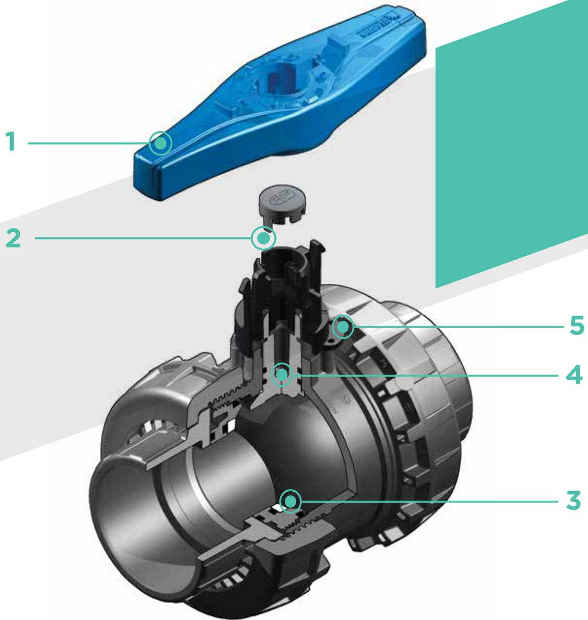
**1 Innovative quick release Easyfit handle** made up of a central hub firmly coupled with the stem by a **dual spoke grip** that can be released from the hub with a simple operation and used as a **ball seat adjustment tool**
