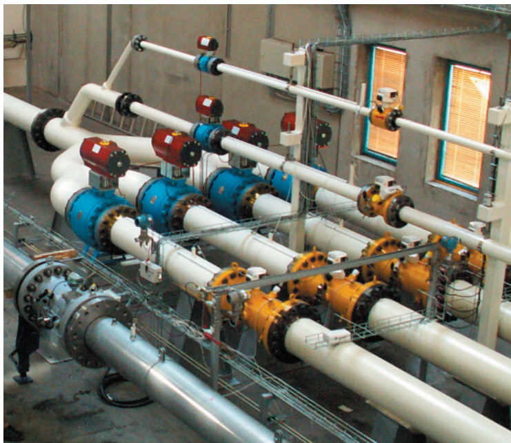
The national reference laboratory Force Technology in Vejen, Denmark. Calibration of gas flow meters.
