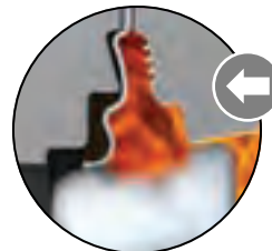
Line pressure applied from non-preferred flow direction. (During or after fire event.)
