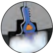
No line pressure. (Pre-fire event condition.)
