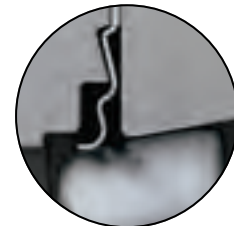
Disc in Closed Position. No line pressure.
